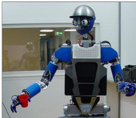
7-DOF arms, and two 5-finger hands, each with tactile sensors and 8 DOFs. ARMAR also includes a number of sensorimotor processes that enable it to act autonomously in complex environments.
