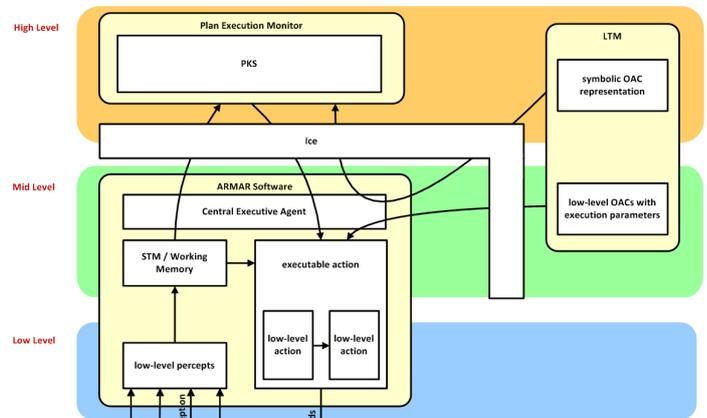
The Ice (Internet Communications Engine) middleware facilitates the exchange of information between system levels/components.
